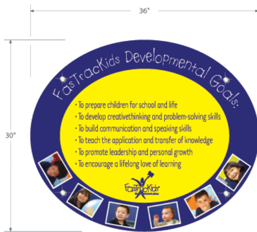
INTERIOR WALL DISPLAY'S SCALE: 1 1/2"-1'-0" FURNISH TWO (2) 30" X 36" OVAL WALL DISPLAY'S. GRAPHICS TO BE OF "C-PRINTS" MOUNTED SECOND SURFACE 1/4" CLEAR PLEXIGLAS. WALL MOUNT W/ ST. STEEL CAP & STANDOFF SYSYTEM.
